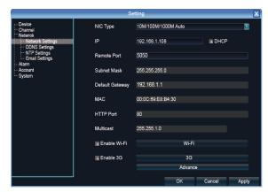
Device port setting: the default is 5050, if there are several NVRs in the LAN, need to change this port is for login NVR by IE, CMS. Login NVR by mobile, the port should be +3 based on the device port.
